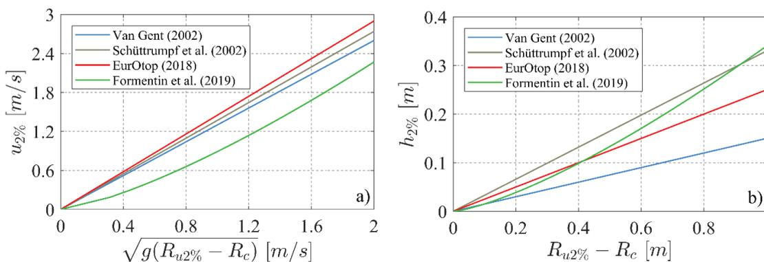
**Figure 1.** Comparison of existing empirical equations for a) overtopping flow velocity and b) layer thickness at smooth slopes; A slope of 1/4 was applied for calculations using EurOtop (2018) equations and Formentin et al. (2019) equations.
