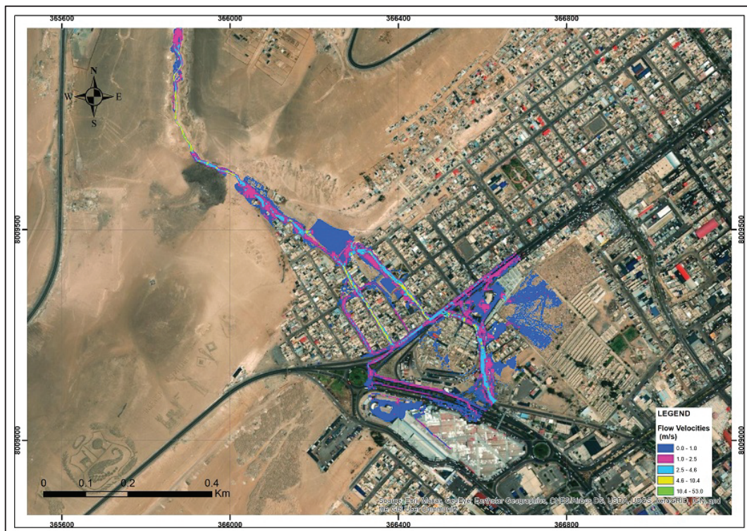
Figure 5. Flow velocities for the "No embankment" scenario.
