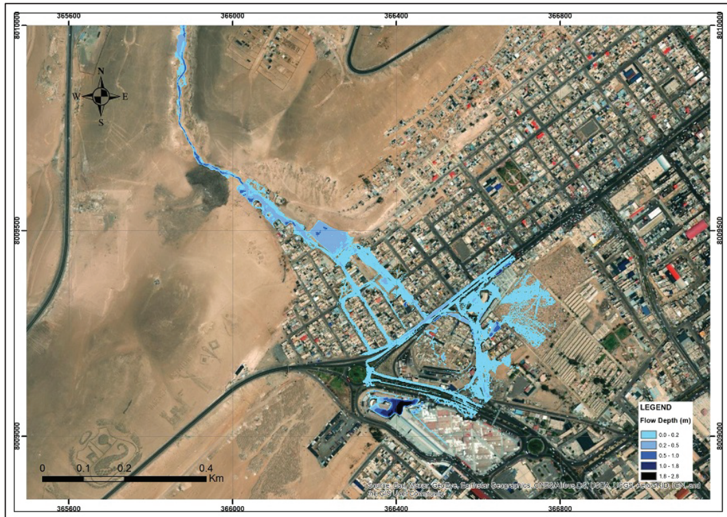
Figure 4. Flow depths for the "No embankment" scenario.
